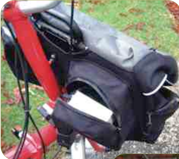
The battery and controller (left) fit easily into a rear pocket of the Brompton pannier, connected by the socket to the motor (Below)
