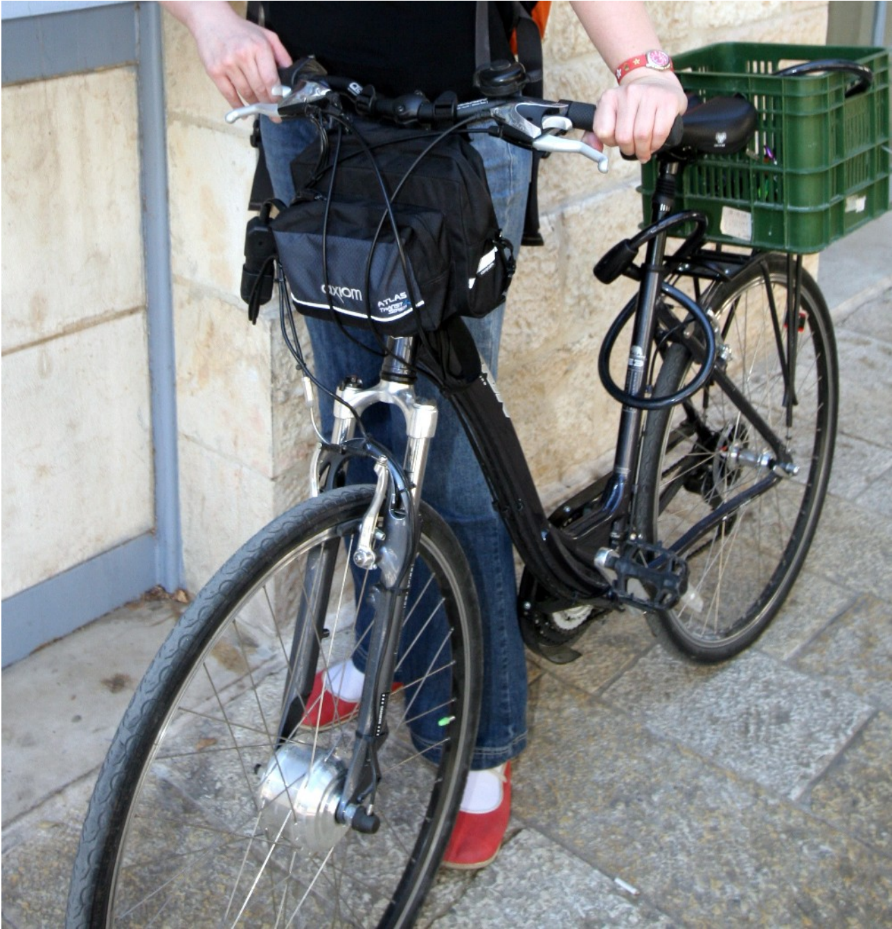
Fitted on 700C city bike with battery in front mounted bag
